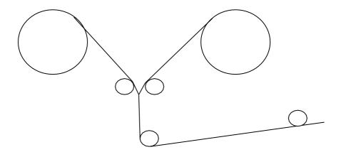
• **Accumulator**: Accumulator consists of number of rollers in series and the fabric is passed over those rollers in order to main constant tension on the fabric and maintain uniform feeding. Top rollers are adjustable and the heights of which is adjusted as per the amount of tension required on the fabric.
