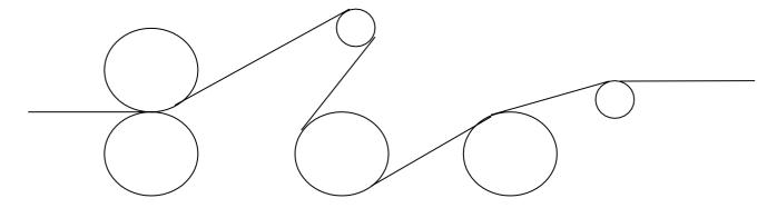
• **Dryer**: The drying of the fabric is carried out on series of cams arranged as shown in fig below:
