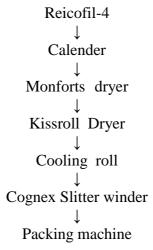
**Line 2**: The fabric produced in Line 1 is taken to Line 2 for further processing in order to giver alchohol repelent finish and vapour cool finish to the fabric. Line 2 is also known as MUCO01. The flow of machines in Line 2 is as followed:
