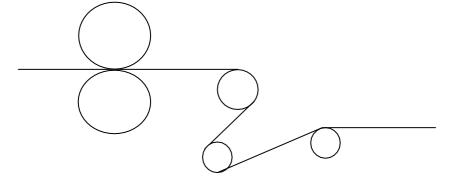
• **Kiss roll**: Kiss roll is a stainless steel roller used for the coating of liquid on one or both sides of the fabric surface. The surface of the roller is friction less and very well polished. There are mainly two kiss rolls provided, the second one is used when the other side has also to be treated. Specifications of kiss roll are:
