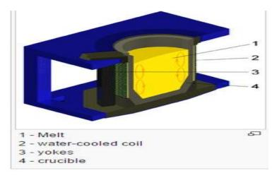
Operating frequencies range from utility frequency (50 or 60 Hz) to 400 kHz or higher, usually depending on the material being melted, the capacity (volume) of the furnace and the melting speed required.
