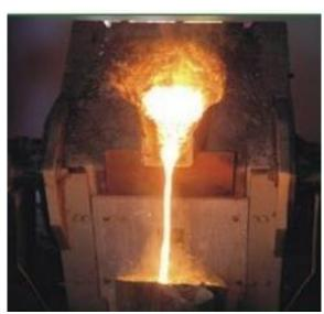
An induction furnace is an electrical furnace in which the heat is applied by induction heating of metal. The advantage of the induction furnace is a clean, energy-efficient and well-controllable melting process compared to most other means of metal melting. Since no arc or combustion is used, the temperature of the material is no higher than required to melt it; this can prevent loss of valuable alloying elements.
