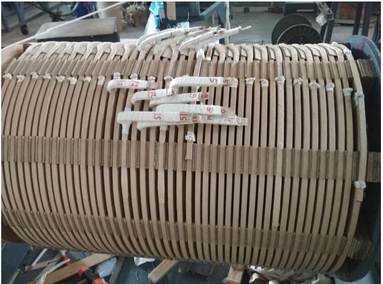
Continuous Disc type winding with tappings
