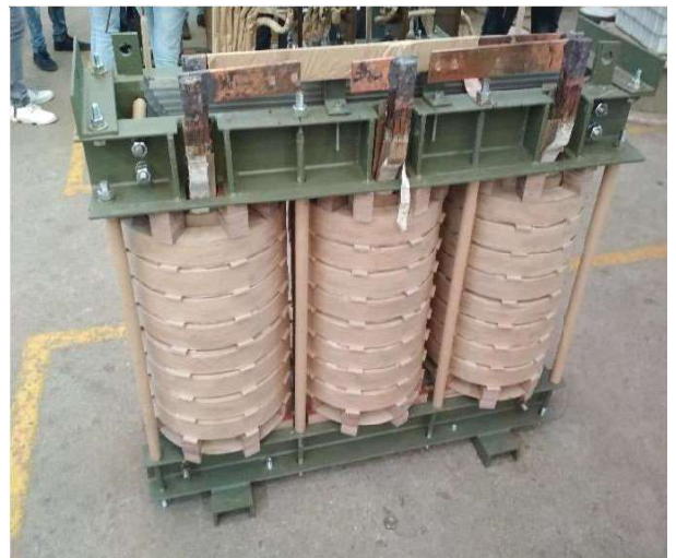
Star Connected Secondary
