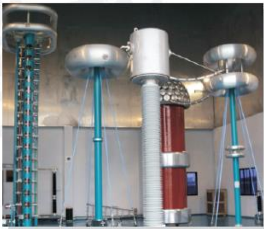
400 kV Current Transformer under High Voltage Test
