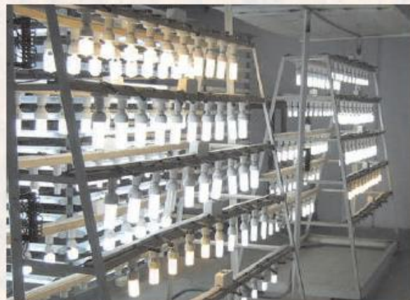
Life test set up for CFL lamps
