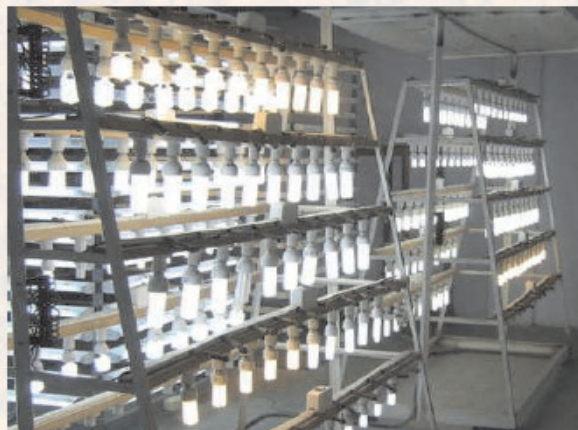
Life test set up for CFL lamps
