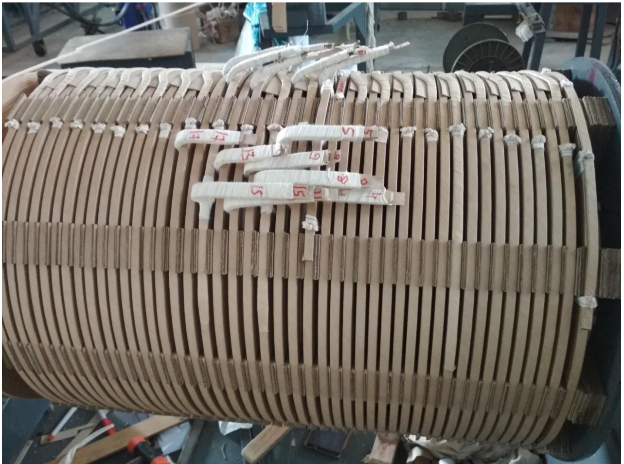
Continuous Disc type winding with tappings
